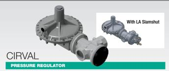
The Cirval is available in two sizes: the Cirval 200 8" head and the Cirval 300 12" head. Pietro Fiorentini's Cirval design is controlled by a diaphragm setting spring, which controls a balanced valve cartridge. Typical applications for the Cirval are medium and low pressure natural gas distribution systems, as well as commercial and industrial applications.
