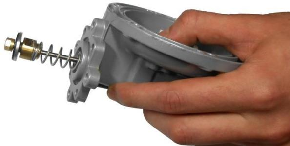
10. Unscrew the nut and remove the obturator
