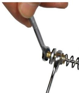
To re-assemble the slam-shut valve, follow the procedure described for disassembly in reverse order. Before reassembling the tightness elements (O-rings, membranes, etc.), it is necessary to check their integrity and, if necessary, replace them.
