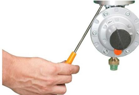
4. Remove the slam-shut device
