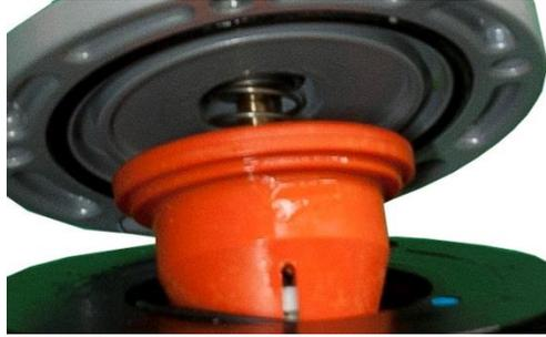
13. Separate the balancing assembly from the head by performing a shift in the gas flow direction so that the stem comes out from the towing coupling;
