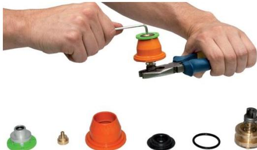
15. Unscrew the valve seat from the body, paying utmost care not to damage the sealing edges;
