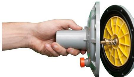
7. Unscrew the nut completely and extract the spring;
