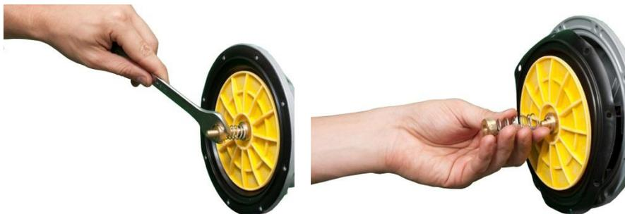
8. Remove the membrane assembly;
