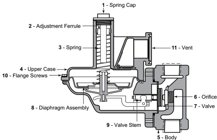
The Model 496 is a general purpose gas pressure regulator for natural gas, air, CO<sub>2</sub>, propane, butane, nitrogen, and other gases. It can be used for gas service to homes, commercial establishments and small industries as well as burners, unit heaters, boilers, and other equipment. All regulators include an internal relief valve.
