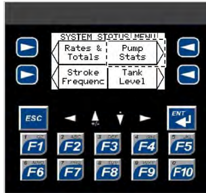
Figure 15: System Status – Pump Stats
