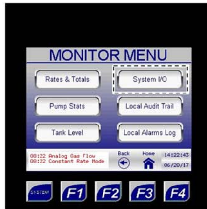
Figure 28: Monitor Menu – System I/O, 2 of 2
