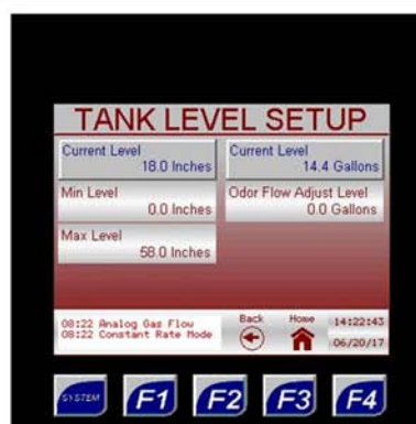
Figure 49: Odorant Tank – Tank Level Setup
