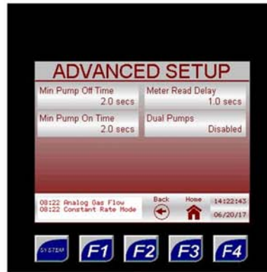
Figure 35: Odorant Pump – Advanced Setup
