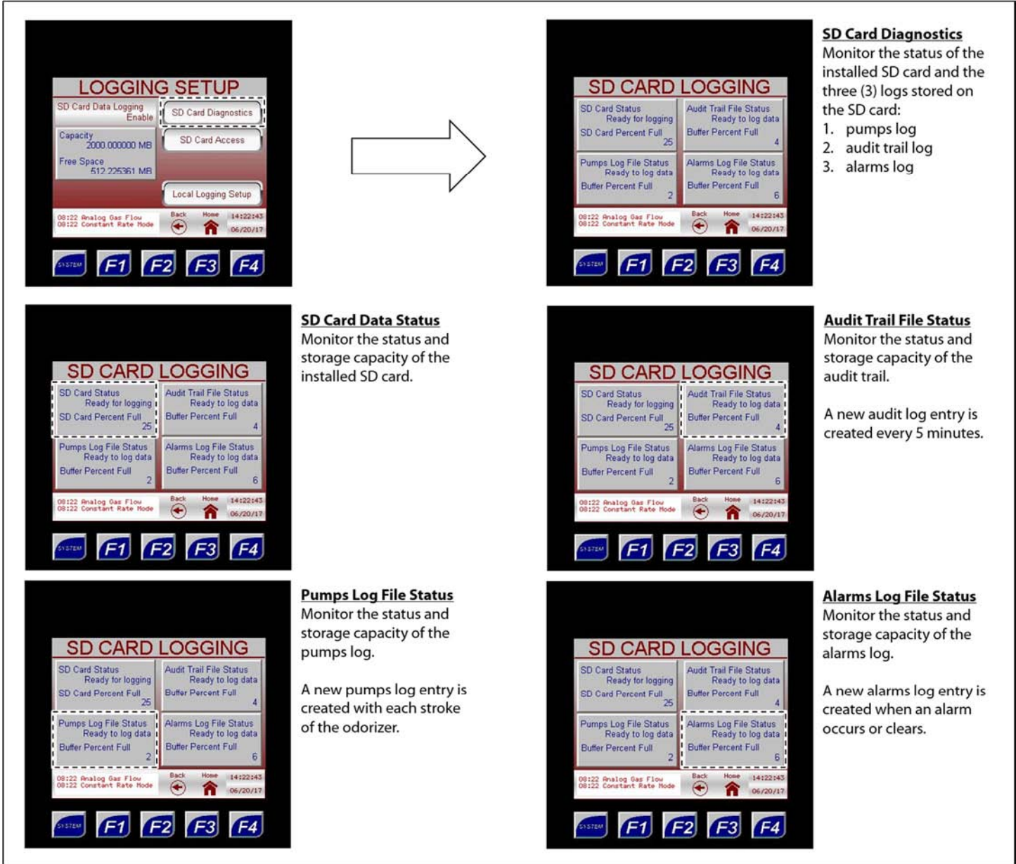
Figure 53: Logging Setup – SD Card Diagnostics
