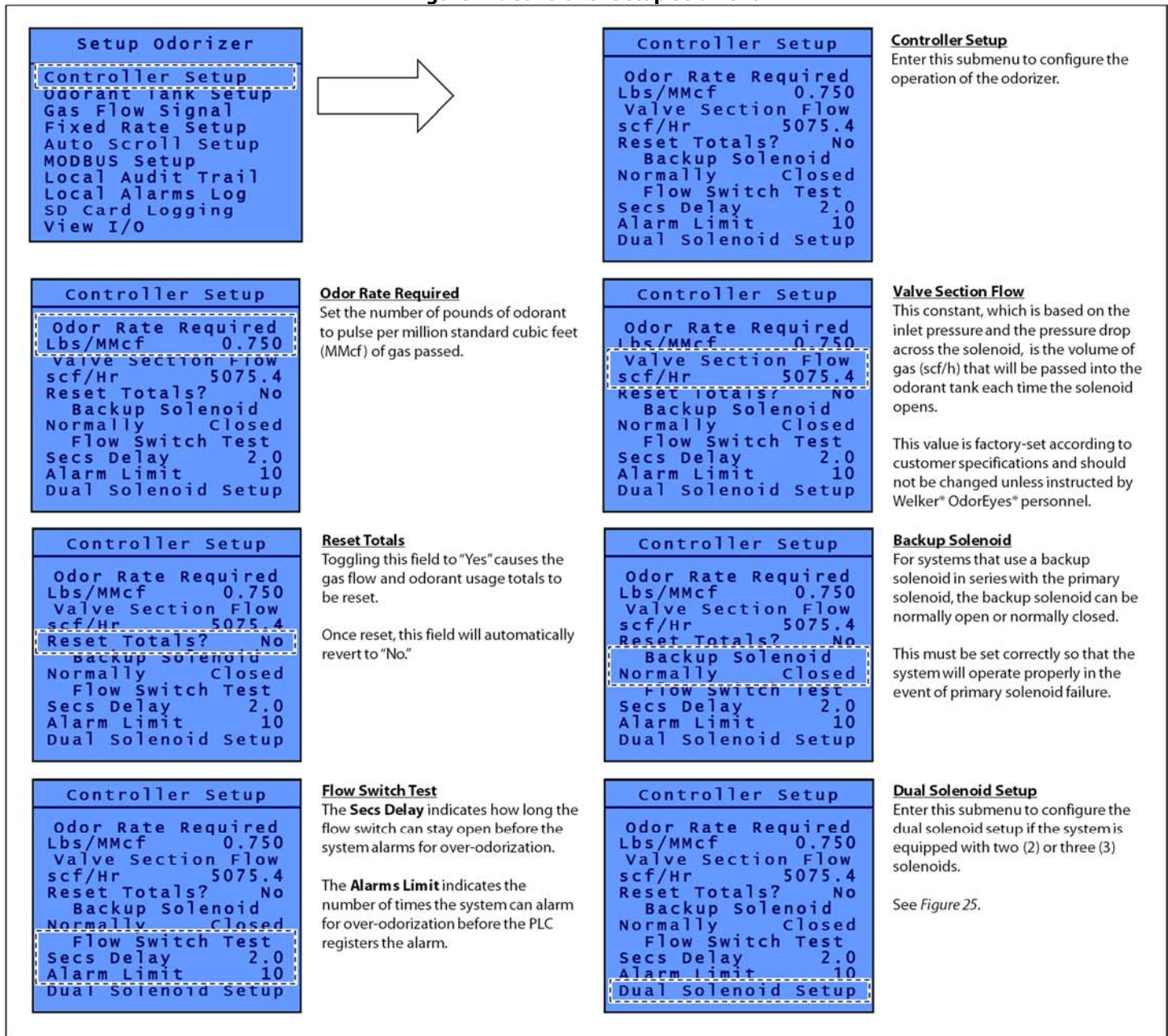
Figure 24: Controller Setup Submenu
