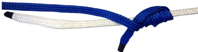
5.4 Take the end of the second rope and wrap around first rope three to six times.
