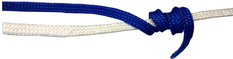
5.3 Bring the end back to the beginning of the knot and place between both ropes.
