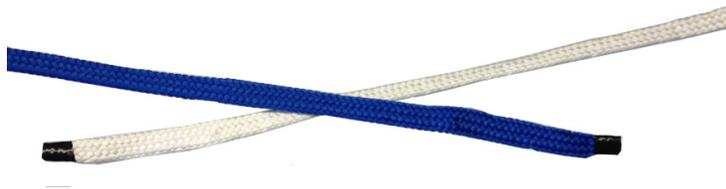
5.2 Take one rope and wrap around the second rope for three to six turns.
